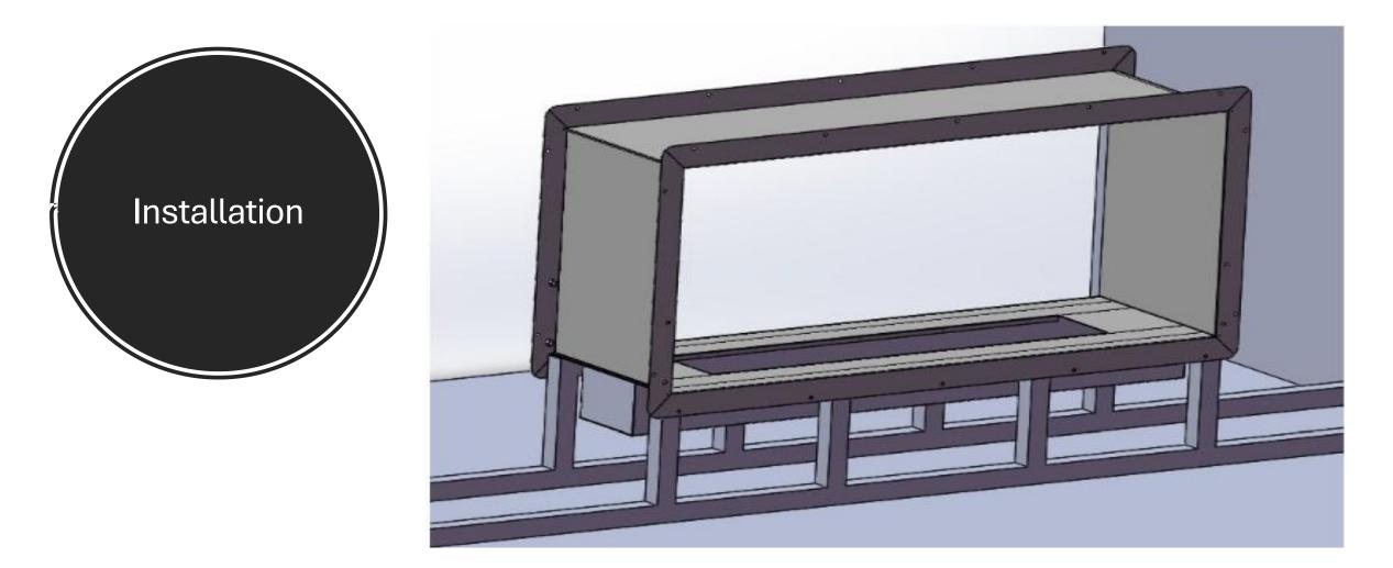
3. Continue building the wall, ensuring that there is a layer of cement board between the stud and your Firebox on all sides.
