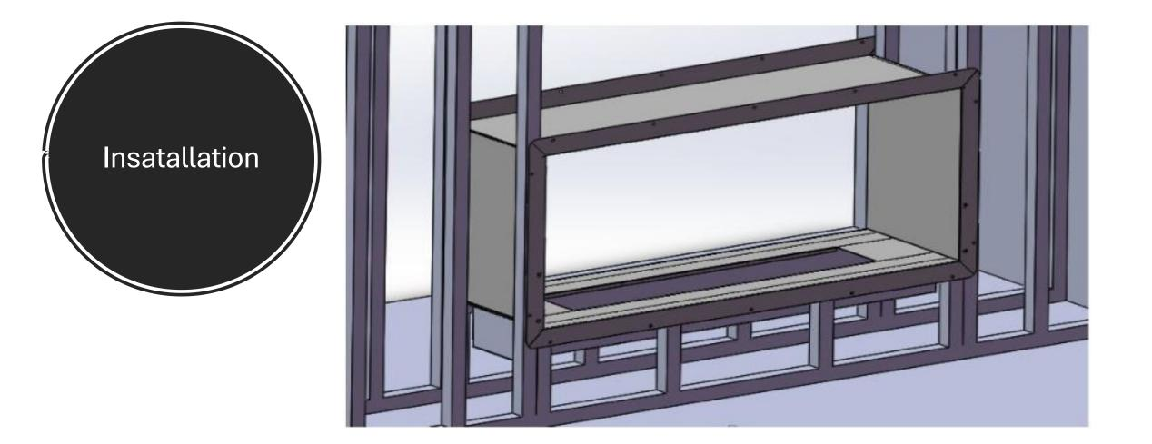
5. Install a stud horizontally on top of the firebox to be able to continue with the wall 6.Screw the top of horizontal stud directly to the Firebox brackets (use 127mm metal zips)
