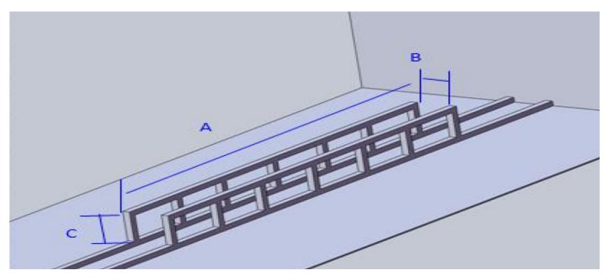
Non combustible materials must be used around the firebox! The Firebox cavity must be a lined with a minimum of 3/8" thick cement board.
