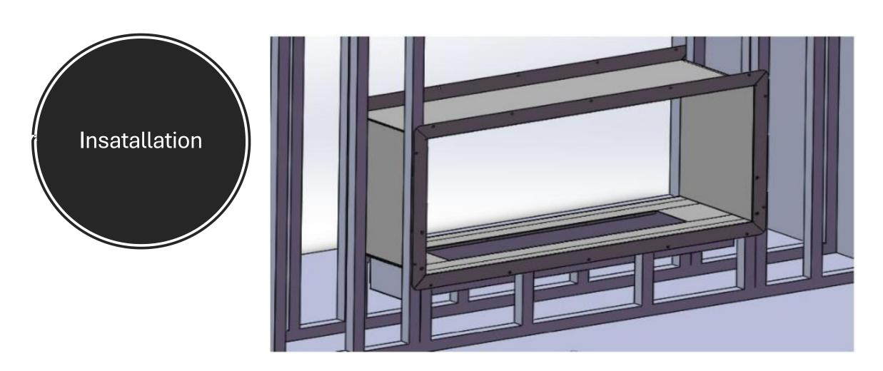
5. Install a stud horizontally on top of the firebox to be able to continue with the wall 6. Screw the top of horizontal stud directly to the Firebox brackets (use 127mm metal zips)
