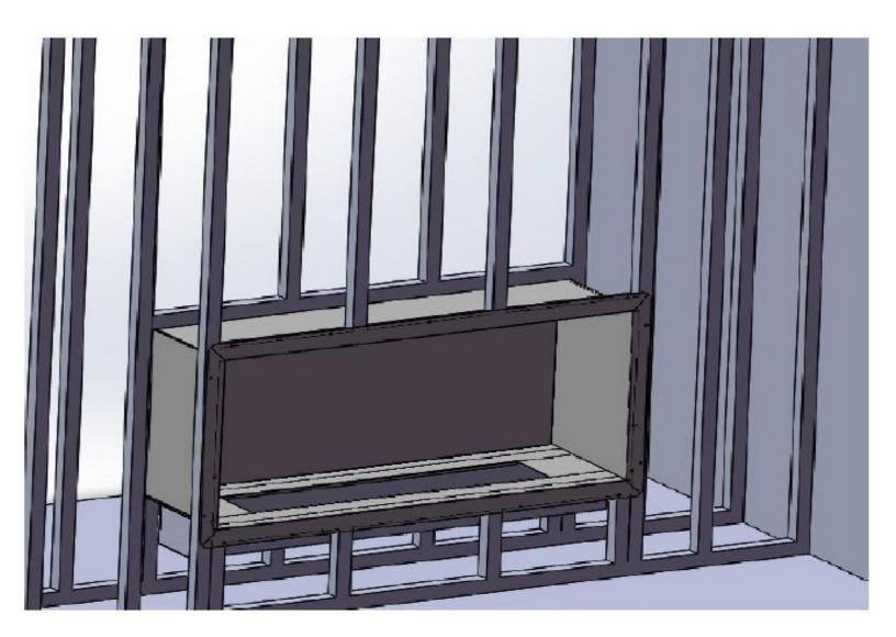
9.Cover the firebox with sheetrock, wonderboard, stones, etc 10.Mount the glass into firebox
