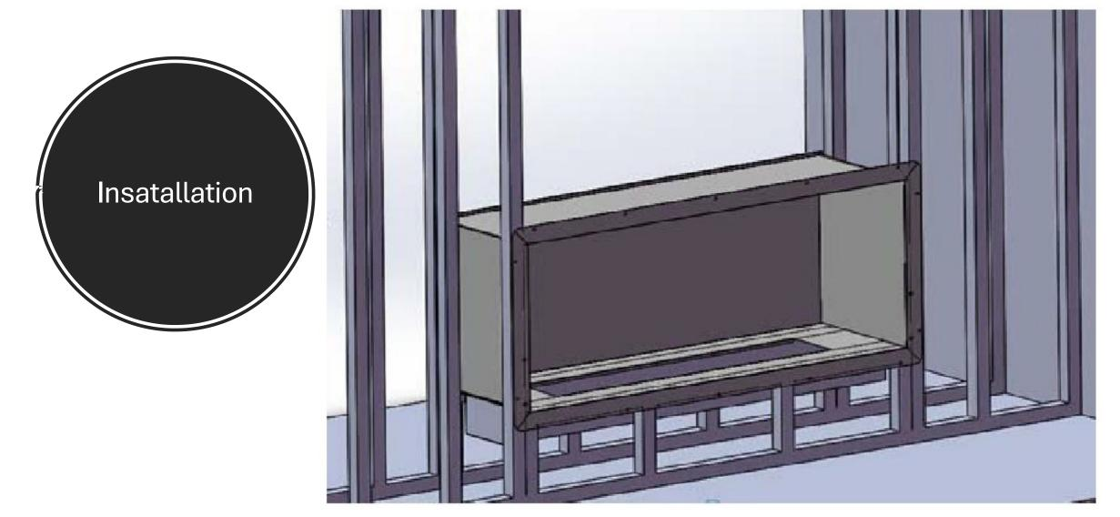
5. Install a stud horizontally on top of the firebox to be able to continue with the wall
