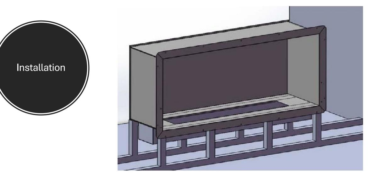
3. Continue building the wall, ensuring that there is a layer of cement board between the stud and your Firebox on all sides.
